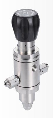
LY RHA two-stage regulator series is designed for use in applications with wide variations between inlet and outlet pressure. In addition, due to the instability of the inlet pressure, the supply-pressure effect will cause unstable delivery pressure. LY two-stage regulator series can minimize this effect and maintain consistent pressure supply.
